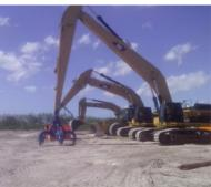
Undercarriage is designed for High-Impact and High-Travel Applications, Like Mining and Heavy Construction. This model is equipped with 900mm tracked shoes.
