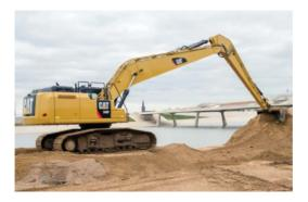
Heavy Duty High Wide (HDHW) Undercarriage is designed for High-Impact and High-Travel Applications, Like Mining and Heavy Construction. This model is equipped with 850mm tracked shoes.
