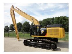
$\label{thm:construction} Under carriage is designed for High-Impact and High-Travel Applications, Like Mining and Heavy Construction. This model is equipped with 900mm tracked shoes.$
