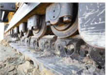
Undercarriage is designed for High-Impact and High-Travel Applications, Like Mining and Heavy Construction. This model is equipped with 700mm tracked shoes.
