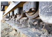
Undercarriage is designed for High-Impact and High-Travel Applications, Like Mining and Heavy Construction. This model is equipped with 1000mm tracked shoes.
