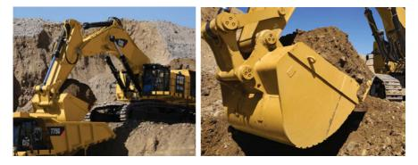
Undercarriage is designed for High-Impact and High-Travel Applications, Like Mining and Heavy Construction. This model is equipped with 1000mm tracked shoes.
