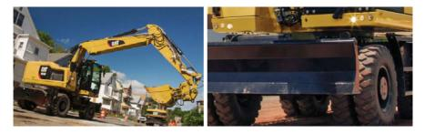
Heavy Duty Axles Long life with effective heavy duty axles. The transmission is mounted directly on the rear axle for protection and optimum ground clearance. The front axle offers wide oscillating and steering angles. Advanced Disc Brake System Minimizes the rocking effect when working free on wheels.
