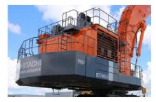
A walkway around the entire counterweight provides easy access for faster, safer inspections and maintenance
