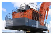
A walkway around the entire counterweight provides easy access for faster, safer inspections and maintenance
